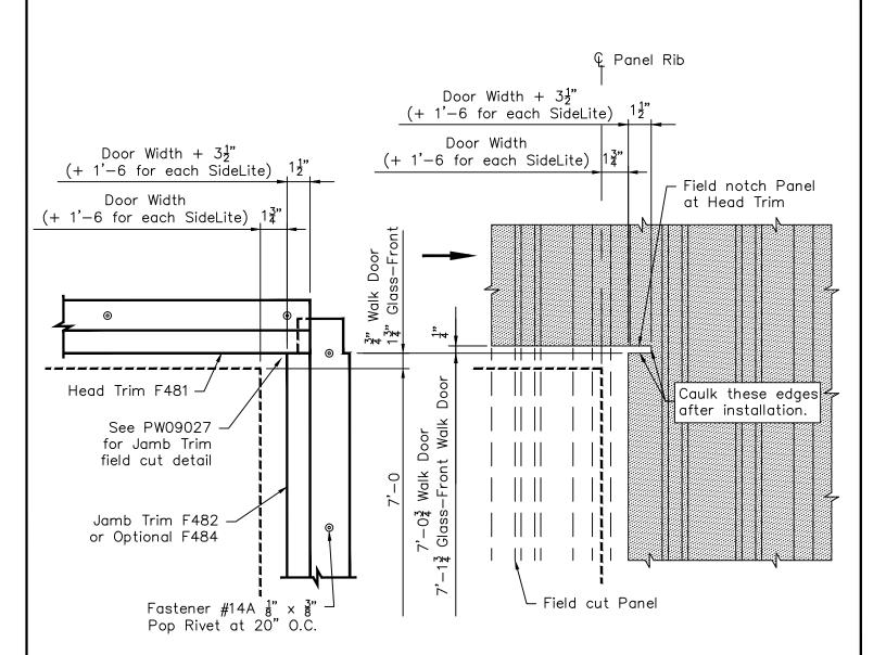
Note: All trim is to be installed BEFORE blanket insulation is applied to walls.
